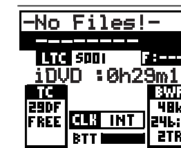
<When the PD-6 internal DVD-RAM drive is selected> iDVD: PD-6 internal DVD-RAM drive
